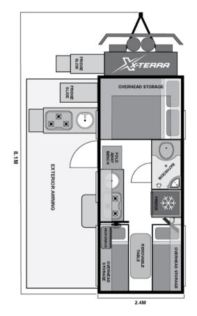
SIZE CLOSED - INCLUDES A/C Length 8.1m - Width 2.4m - Height 3.1m
