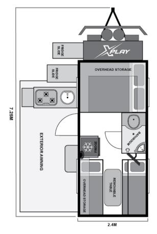
SIZE CLOSED - INCLUDES A/C Length 7.25m - Width 2.4m - Height 3.1m
