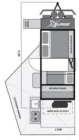
SIZE CLOSED - INCLUDES A/C Length 6.2m - Width 2.25m - Height 2.45m
