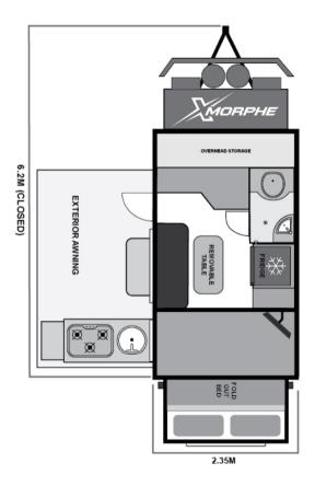
SIZE CLOSED - INCLUDES A/C Length 6.2m - Width 2.3m - Height 2.8m
